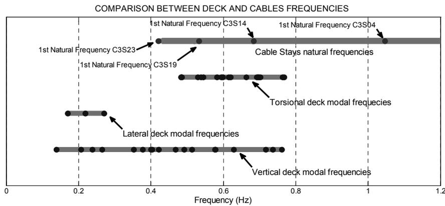
Figure 2. Comparison of deck with 1<sup>st</sup> cable stay frequencies
