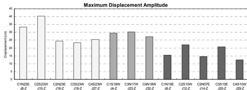
Figure 15. Maximum displacement amplitude of cable stays sorted per length
