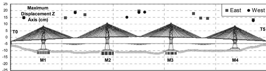
*Figure 13.* Maximum vertical displacement amplitude at sensor location
