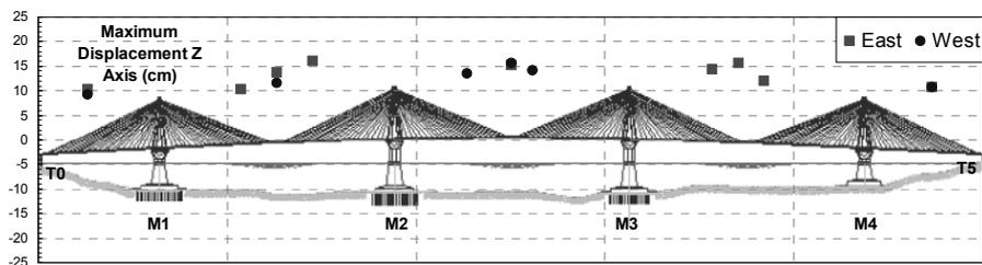
*Figure 6.* Maximum vertical displacement amplitude at sensors location
