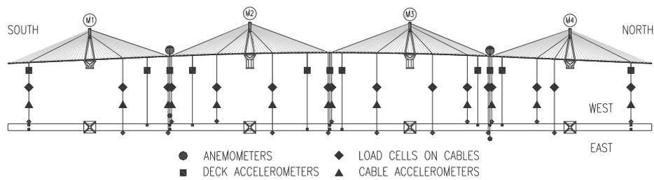
Figure 4. Location of structural monitoring sensors (cable relevant)
