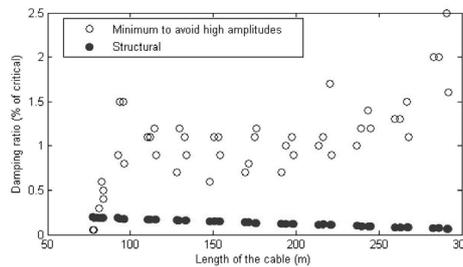
Figure 9. Required damping ratio for vibration mitigation
