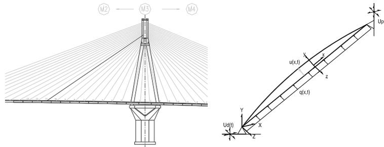
Figure 3. Configuration model for cable response calculation
