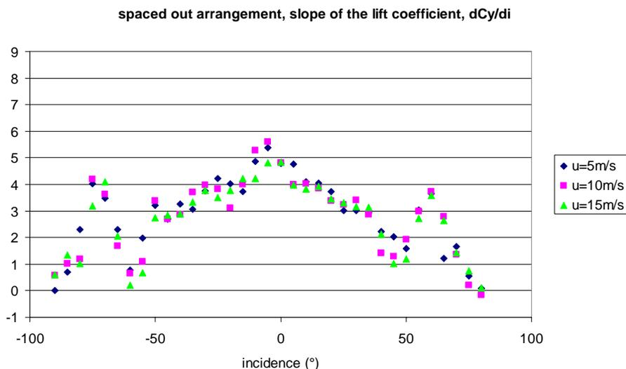
Figure 11 :Spaced out arrangement,  $C_y$  coefficient slope variation with wind incidence
