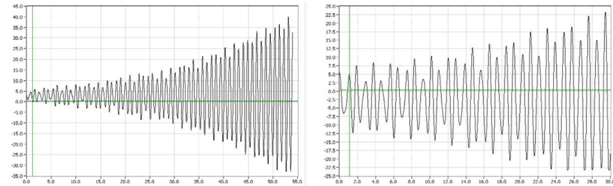
Figure 14 : increasing amplitude of compact arrangement cable for wind speed 5m/s at incidence  $54^\circ$  (left) and  $1^\circ$  (right).
