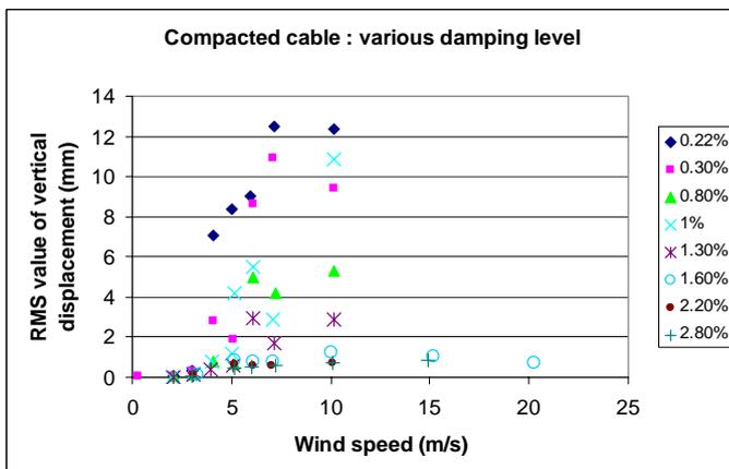
Figure 15 : Effect of increasing structural damping on galloping amplitude of compact arrangement cable.
