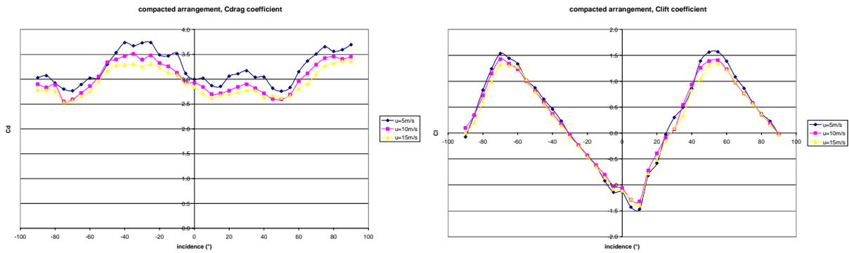
Figure 7 : Compacted arrangement, Cd drag coefficient (left) and Clift coefficient (right) for wind incidence varying from -90° to +90°
