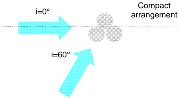
Figure 12 : Coordinates for dynamic testing of compact arrangement of ropes
