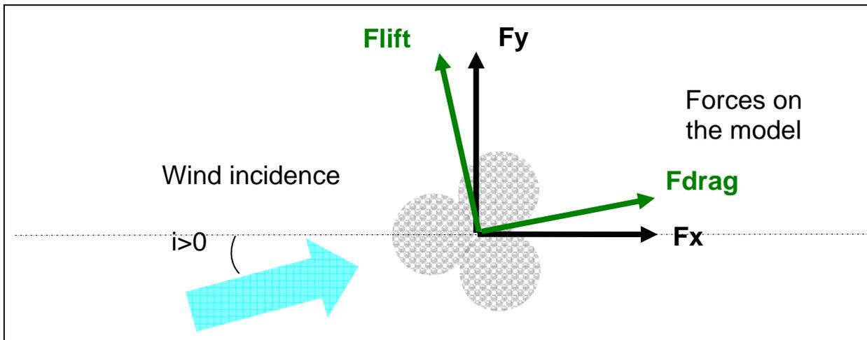
Figure 6 : force coefficients coordinates for compacted arrangement study
