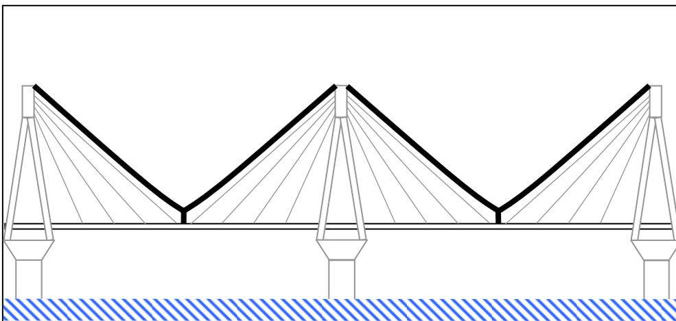
Figure 1 : principle of the stretch cables protecting Rion-Antirion bridge stays from lightning
