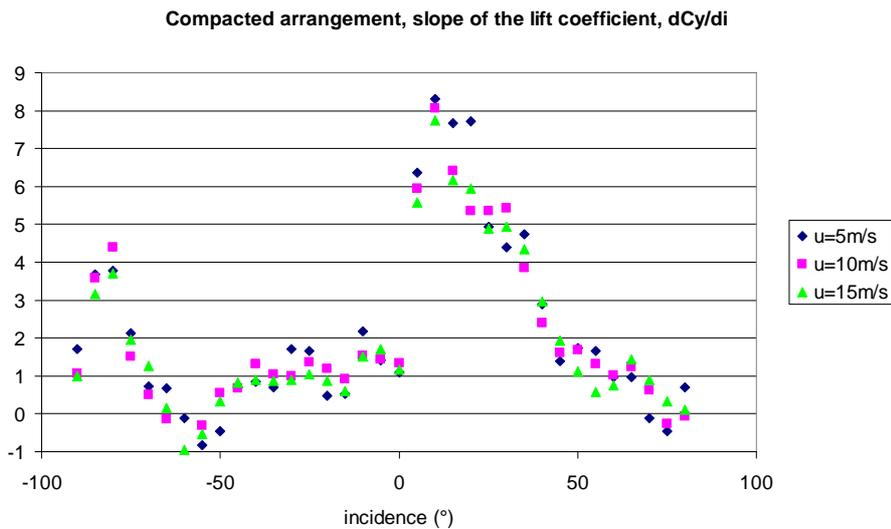
Figure 8 :Compacted arrangement,  $C_y$  coefficient slope variation with wind incidence
