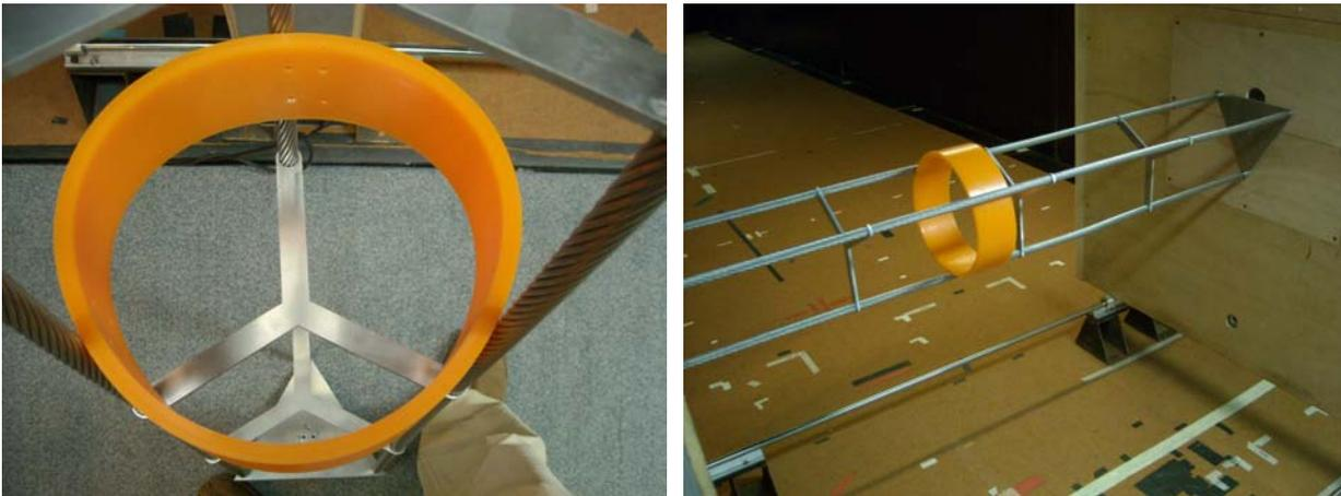
Figure 16 : Wind tunnel test of spaced out cable stability when equipped with a PU ring acting as a damping spacer.
