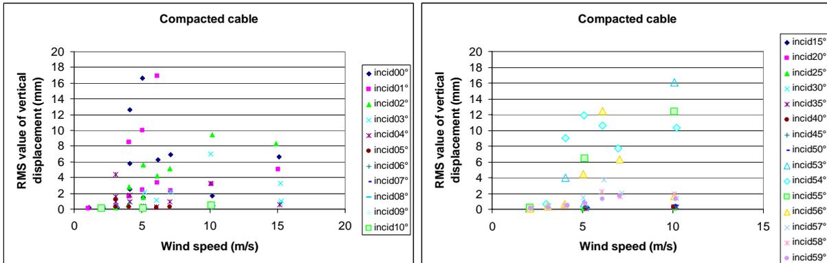
Figure 13 : Aeroelastic response of compact arrangement cable with wind speed, amplitude in mm.
