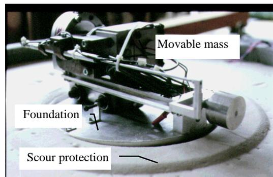
Figure 3. Model foundation (scale 1/100)
