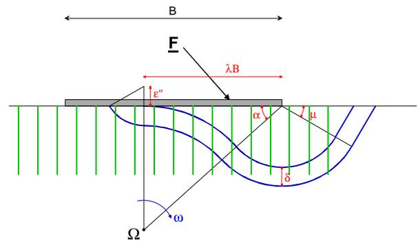
Figure 13. Kinematic mechanism
