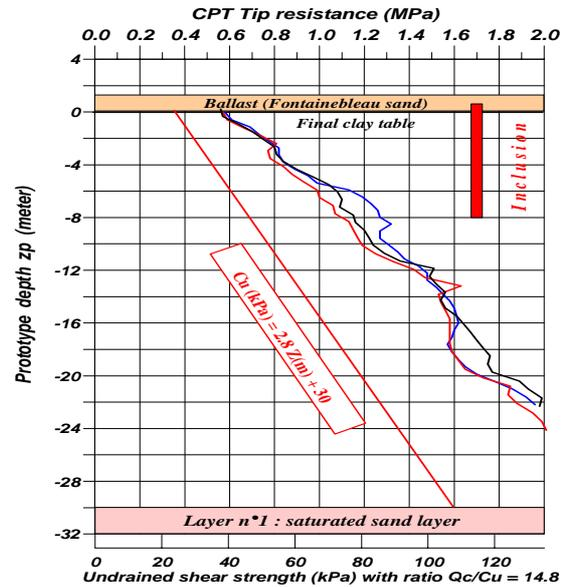
Figure 6. Shear strength profiles from in flight CPT tests performed into the clay sample (Test 2)
