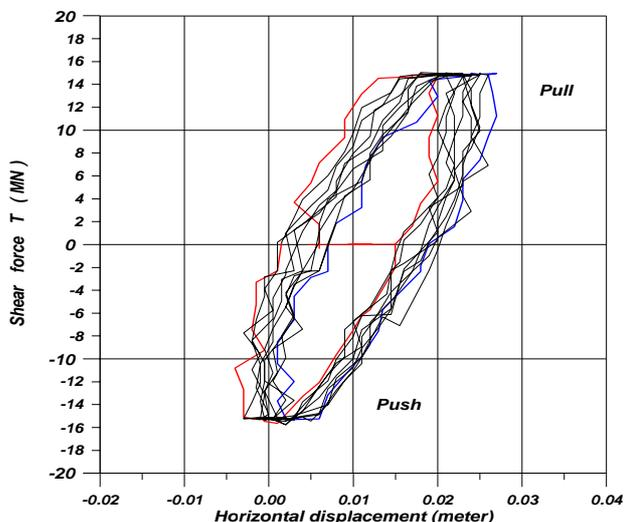
Figure 8. Test 2 : Horizontal displacement of the foundation vs. cyclic shear force T (sequence 2)
