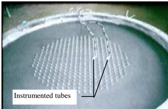
Figure 4. Inclusions jacked into the clay bed
