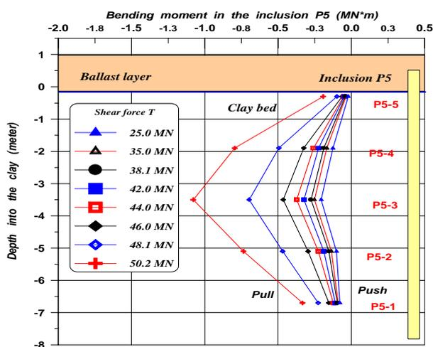
Figure 10. Test 2 : Bending moment vs. depth in inclusion P5 during loading sequence 5
