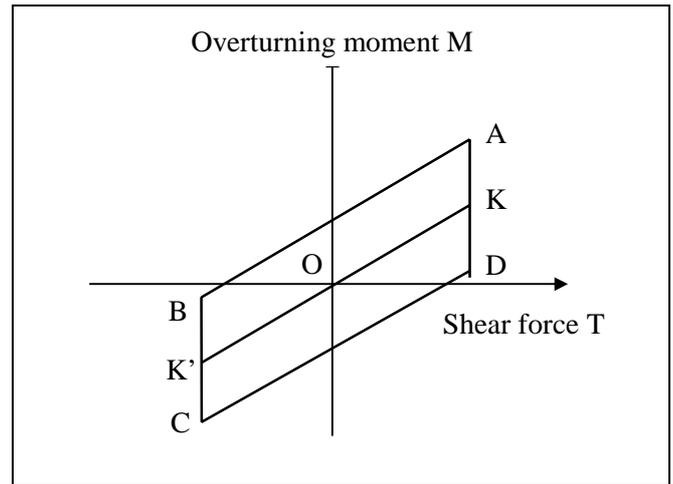
Figure 5. Typical load path
