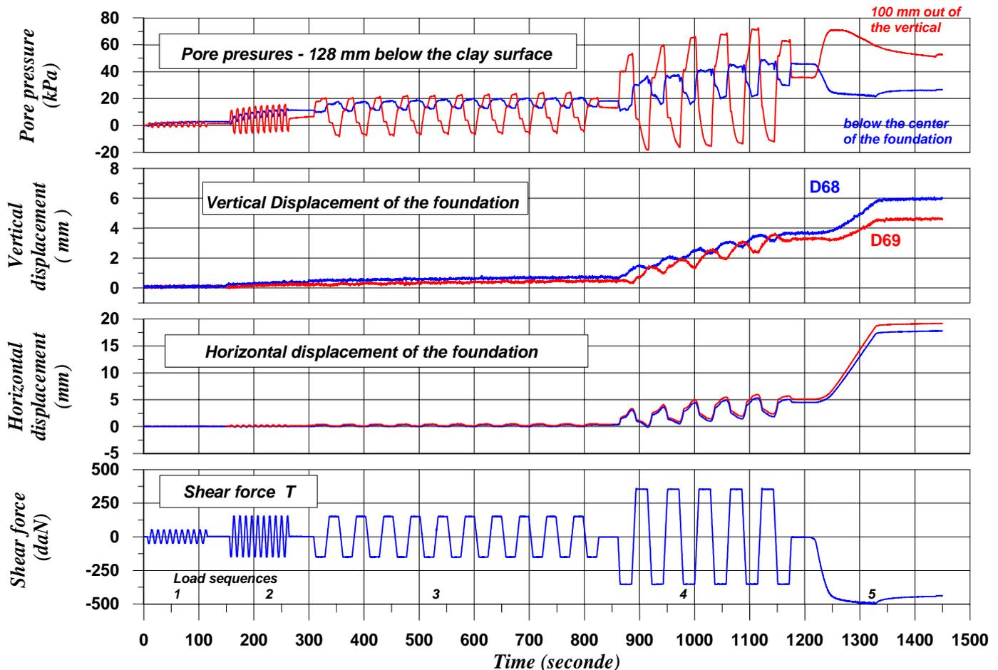
Figure 7. Test 2: horizontal load T, vertical and horizontal foundation displacements, pore pressure vs. time in model conditions.
