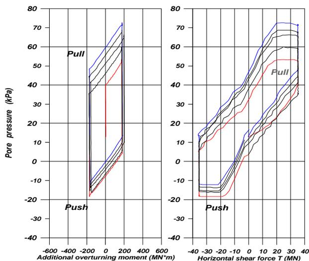
Figure 9. Test 2: Excess of pore pressure due to cyclic loading 12.8 m deep in the clay and 10 m
