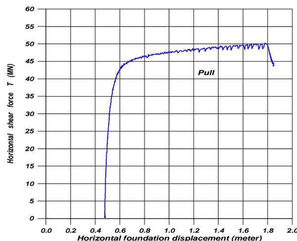
Figure 11: Test 2: Horizontal shear force vs. foundation displacement in loading sequence 5
