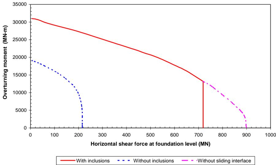
Figure 4. Bounding surface for a reinforced soil.
