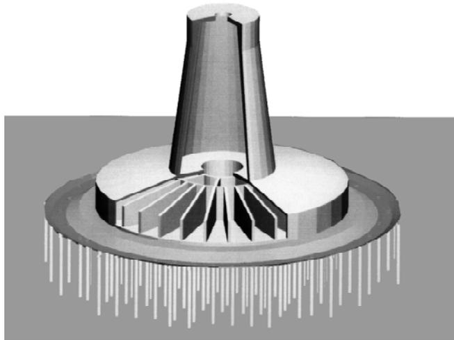
Figure 3. View of a reinforced soil foundation (Dumez-GTM).
