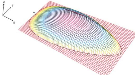
Figure 2. Skeletal view of the bounding surface for a cohesive soil without tensile strength.
