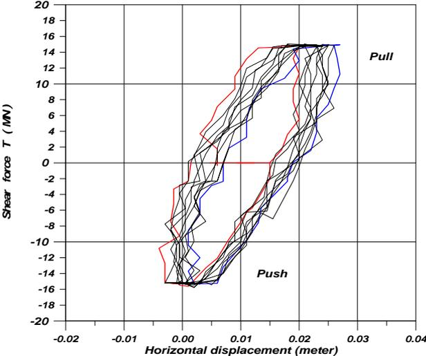
Figure 7. Horizontal displacement of the foundation vs. cyclic shear force T.
