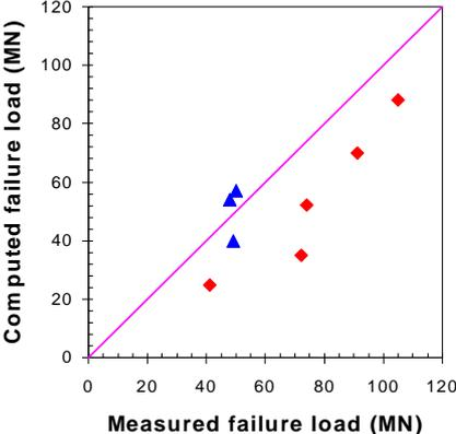
Figure 6. Comparison between measured and computed ultimate loads.
