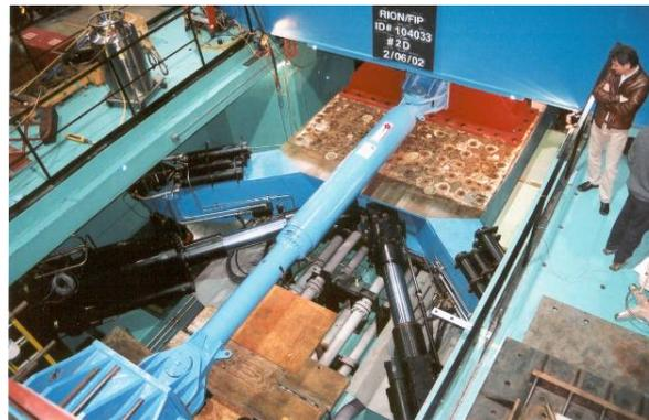
Fig. 9 Prototype testing of hydraulic dampers at SRMD Facility (UCSD)
